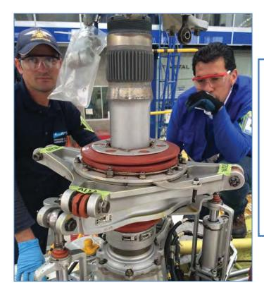
Excessive roughness detected on Swashplate Assy Duplex Bearing P/N 109-0101-21-1.
