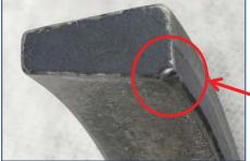
Damage on Lower Conical ring set P/N 109-0101-21-1 S/N A0128, replacement required
