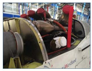
General Visual Inspection TRDS, TGB & T/R Rotating Controls without discrepancies noted. Also borescope inspection was performed inside the Tailboom, torque check to Fuselage-Tailboom attachment bolts with satisfactory results.
