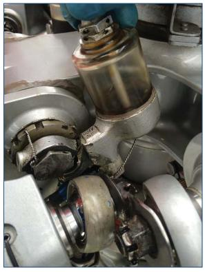
Additional, this impact moves the Oil reservoir assy upward hitting the Fairing Cover P/N 109-0855-40-101
